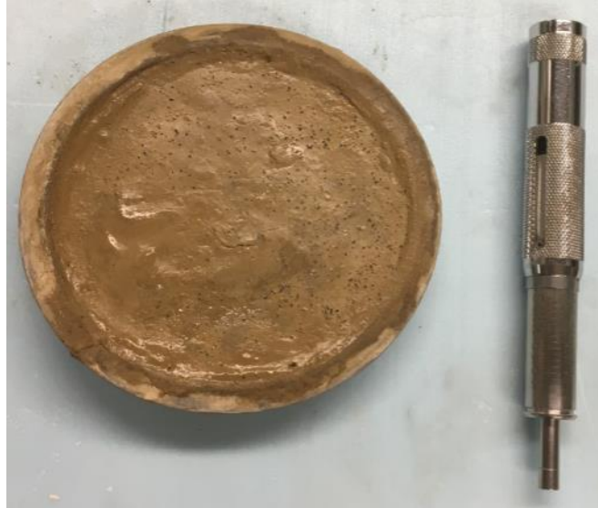
Figure 1. Setting time apparatus: Pan (left) and penetrometer (right)
